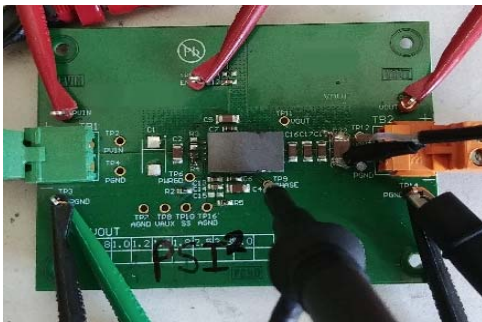
Fig. 5. PSI 2 module mounted to testing board.
